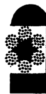
RIGHT WAY Always measure the larger dimension, between the outer limits of the strands
