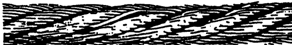
Improper handling. Kink or "dog leg" was caused by improper handling and/or installation. A kink causes excessive localized or spot abrasion.
