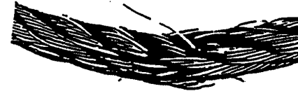
Reverse bending. Running this rope over one sheave caused fatigue breaks in wires.
