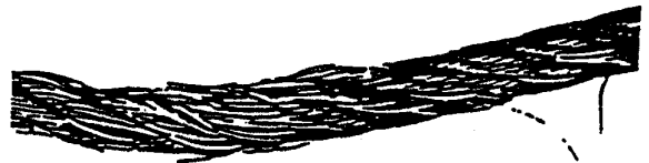
Undersize sheave grooves. Sheaves were too small, causing strands to pinch. Wires then fall in the valley between the strands.
