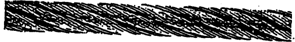
Excessive exposure to elements. Too much exposure combined with surface wear and loss of lubrication caused corrosion and pitting.
