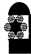
WRONG WAY Do not measure the smaller dimension across the "flats" of the strands.
