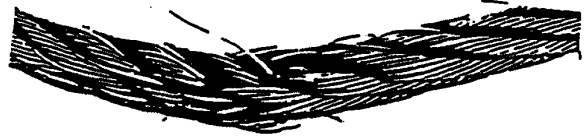
Reverse bending. Running this rope over one sheave and under another caused fatigue breaks in wires.
