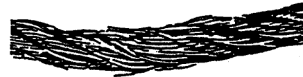
Undersize sheave grooves. Sheaves were too small to pinch. Wires then fall in the valley between the strands.
