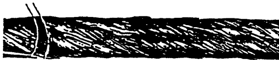
Infrequent inspection. Neglect of periodical inspection left this rope in service too long, resulting in considerable abrasion.
