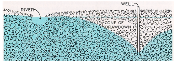
Figure 27b. Well located away from the river removes water from storage.
