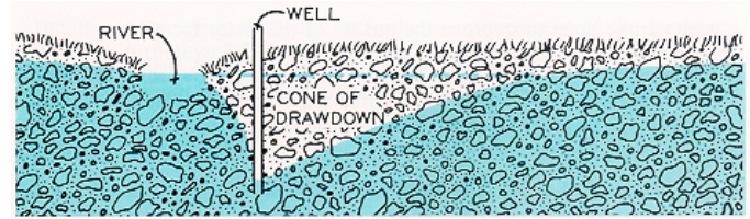
Figure 27a. Well near the bank draws water from the stream.
