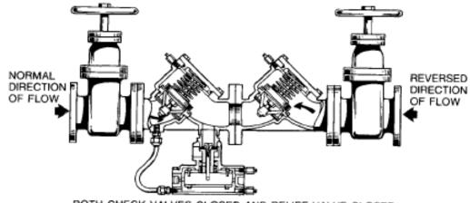
BOTH CHECK VALVES CLOSED AND RELIEF VALVE CLOSED
