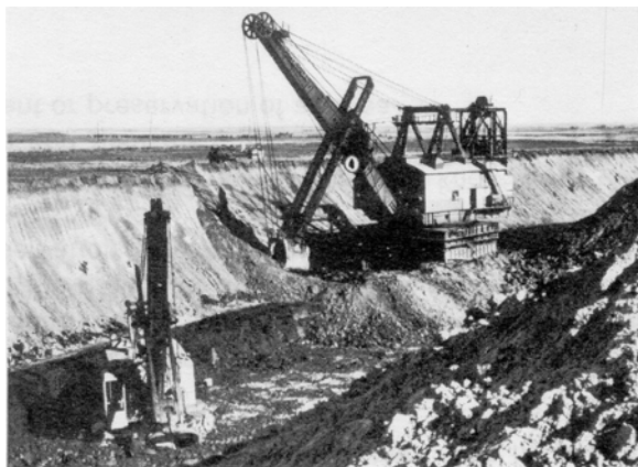
Strip mining lignite at the Velva mine near Velva, North Dakota. The large 22-yard shovel is removing overburden; the smaller shovel is mining lignite.
