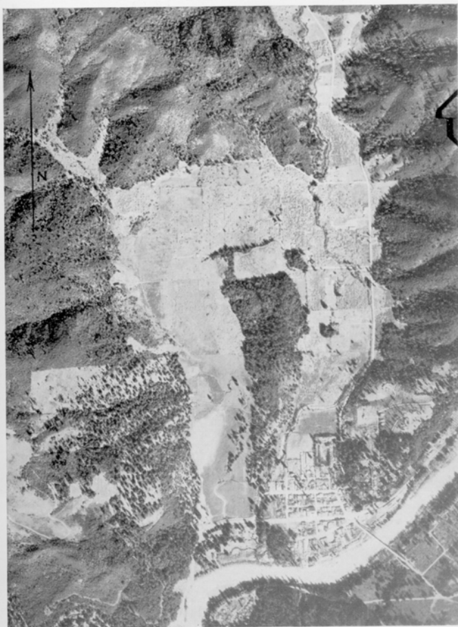
Aerial photograph of abandoned entrenched loop of the Russian River north of Guerneville, California. Scale: one inch equals approximately 1,800 feet. The small streams draining the loop are clearly incapable of having eroded it
