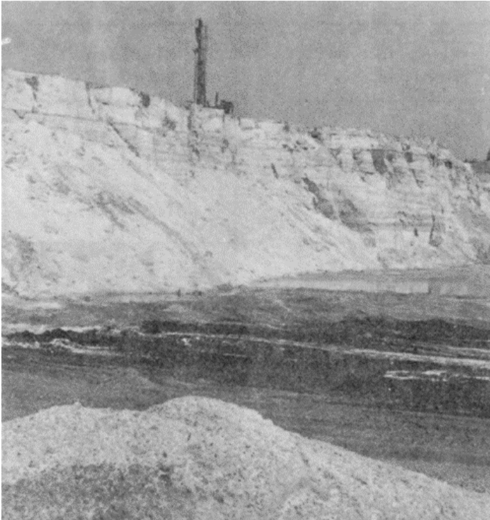
Figure 6. Operations. of the Ottawa Silica Co., Rockwood. Blasted sand from face on center and left. Drill on stripped, upper bench.
