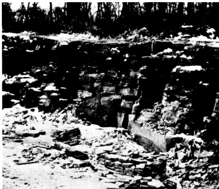
Figure 17. Quarry face, Napoleon Sandstone, showing slabby separation planes, Napoleon.
