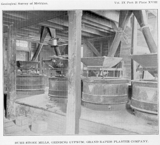
[XVIII. Buhr Stone Mills Grinding Gypsum; Grand Rapids Plaster Co.]
