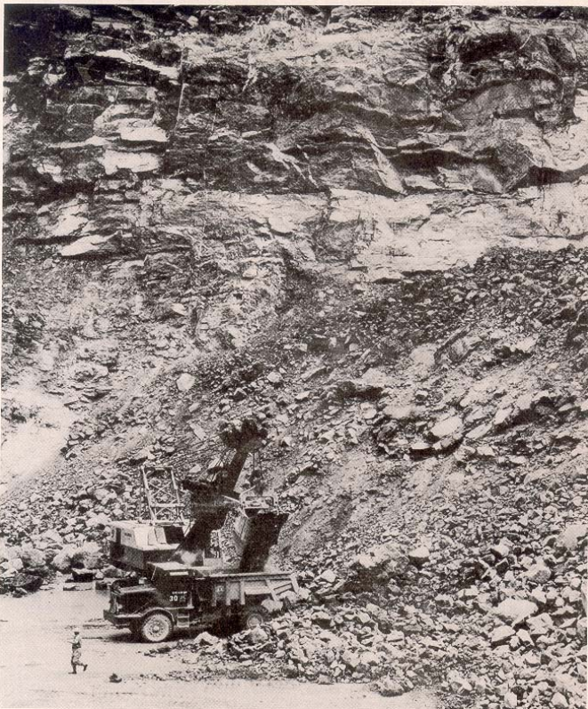
Figure 2. - Limestone is scooped from the quarry floor into a 22-ton truck by power shovel at Jones and Laughlin Steel Co. quarry in West Virginia.
