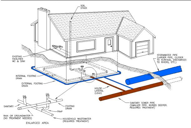
**Diagram of a Footing Drain Connected to the Sanitary Sewer System**
