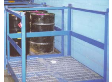
Example of using racks to protect drums from physical damage from traffic.
