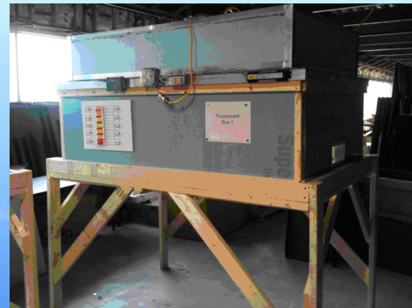
Lamps run continuously on a 3-hour on, 20-minute off cycle at 45°C inside of temperature control chambers
