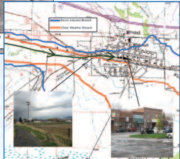
FIGURE 3: Debris may force the breach flow outside of the clear weather breach boundary.
