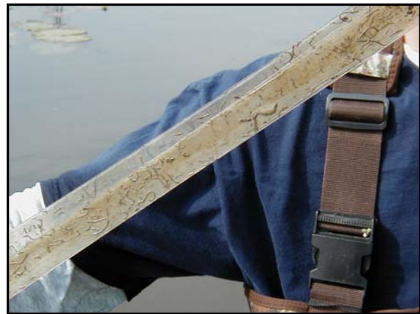
Figure 2.2. SPMD and Biofouling
