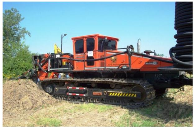
**Bron tile drainage machine used for installation. GPS is used to steer and control grade.**
