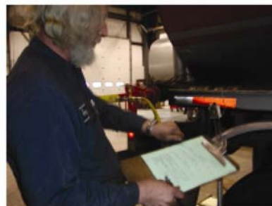
FIGURE 11. Pressure/vacuum tests conducted on a tanker truck.
