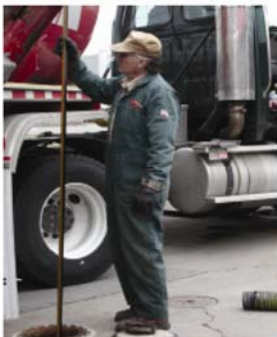
FIGURE 7. Sticking a tank to verify the tank's fuel capacity.
