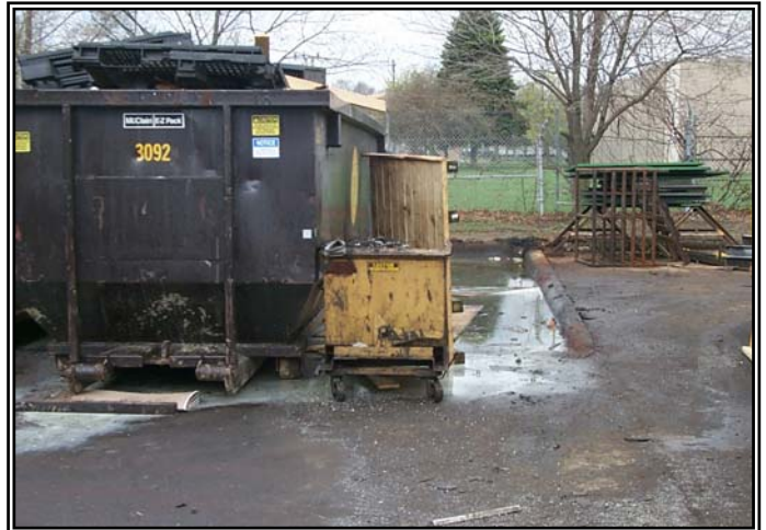
Improper storage and disposal of wastes and polluting materials at commercial and industrial facilities can pollute local storm drains.
