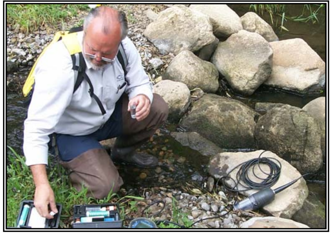
Water quality testing for pollutants associated with illicit discharge sources is performed.
