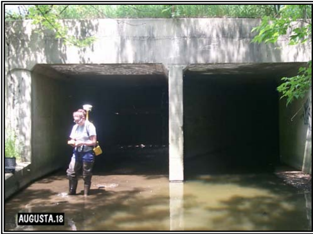
Surveys are done to locate and examine outfalls from county drains for signs of pollution.
