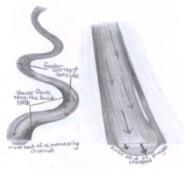
**Figure 6: Natural Channel vs. Straightened/Dredged Channel**
