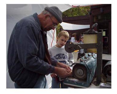
Using lapidary equipment to grind, shape and polish.
