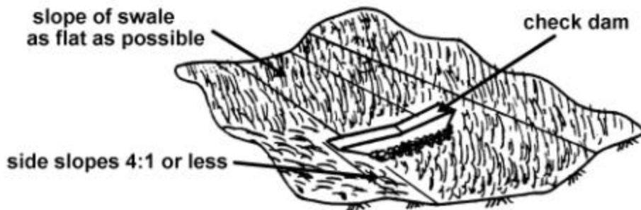
Figure 5.3 - Grassed Swale with Check Dam
