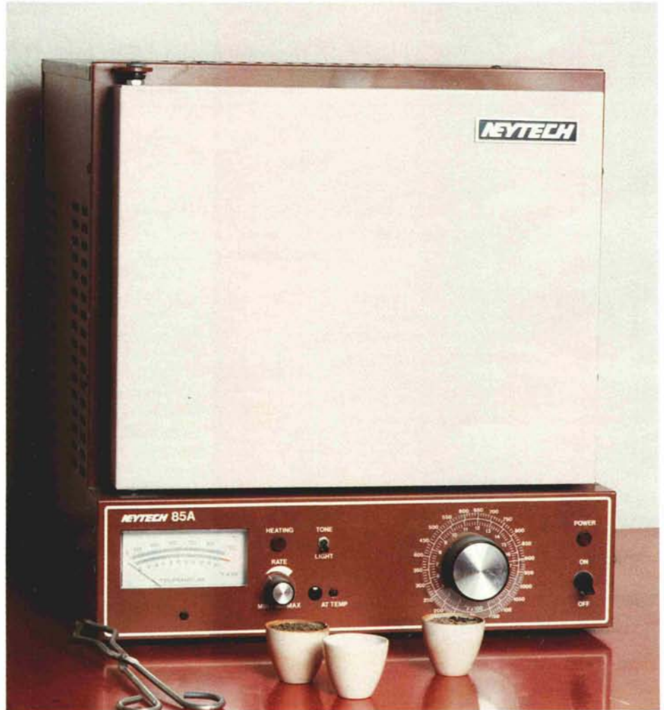
A muffle furnace, used for organic matter analysis.
