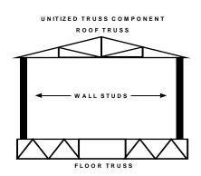
The next generation of truss construction may very well use a process called "unitized trusses" to construct buildings. The unitized truss concept incorporates the truss roof rafter, the wall stud, and the truss floor joist built and installed as one integral unit. This method would work best for trusses built and installed at the construction site, due to the size of the completed unitized
