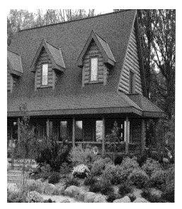
Log construction is the most basic of wood-frame construction As the early settlers methods. cleared the land of timber, the smaller logs were used to construct buildings by placing them one on top of another. They were fastened with a self-locking technique where the ends would be notched to interface with a notch from a second log at a 90-degree angle. With the limited availability of tools, mainly using an axe, the settlers could fashion a building from the logs quickly and easily.
