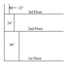
Bearing walls carry the load of the structure, which is transferred to the wall from the floor joists and roof rafters. Failure of a load-bearing wall can result in catastrophic structural collapse. It is critical that all emergency scene personnel be able to identify the load-bearing walls and understand the dangers associated with wall failure. Bearing walls are typically the longest walls of the structure. This may be the front (street side) or, most
