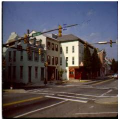
Other common terms applied to Type III or ordinary construction are USA," "Main Street and "Taxpayer." The term "Taxpayer" evolved from "Main Street USA," where a building owner would operate a retail store on the first floor and live in an apartment on the second floor. It was said that the property taxes for the building were paid for by the store's income, and the shop owner lived above the store tax free.
