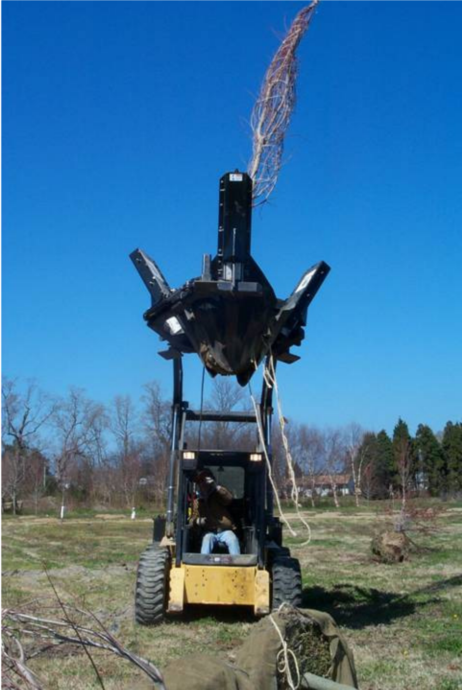
Figure 5. Dormant field-grown tree lifted into air to be dropped to bare root the tree.
