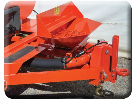
Hitch adjusts for height and distance
