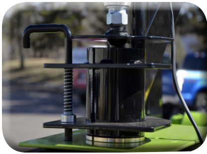
Stress-free boom rotates around hose
