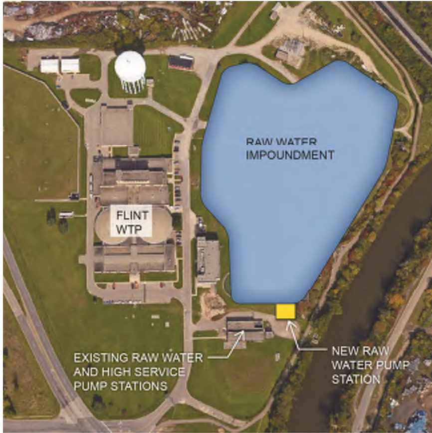
Figure 3.3 – Earthen Berm Impoundment Plan View
