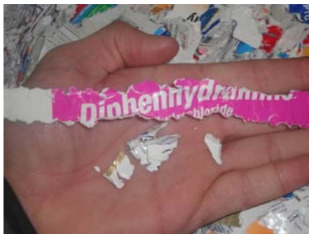
strip cut shred compared to grinder shred
