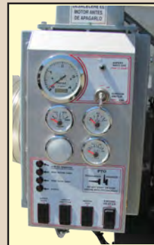
Hinged instrument panel allows easy access to the instrument wiring. All engine monitoring gauges are backlit for increased visibility. Gauges and controls include: throttle control, tachometer, hour meter, oil pressure, water temperature, volt meter and fuel gauge.
