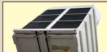
Vented top screens are located on top of the unit for proper air flow. These screens are made of 1/2" expanded steel with mesh screen. They are easily removable and slide in and out on channels. (Unit shown with optional color)
