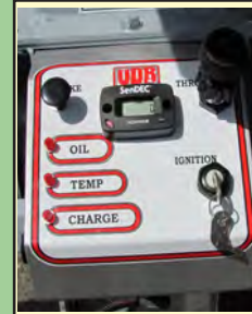
Engine controls and gauges include: tachometer, hour meter, throttle, choke and keyed ignition switch. Indicator lights for low oil pressure, high engine temperature and battery charging are included.
