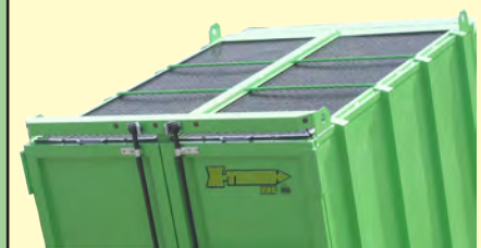
Vented top screens are located on top of the unit for proper air flow. These screens are made of 1/2" expanded steel with mesh screen. They are easily removable and slide in and out on channels. (Unit shown with optional color)
