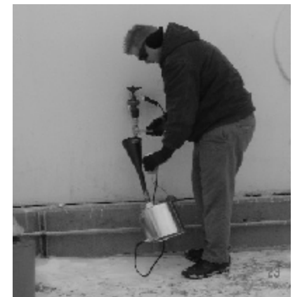
A field metrologist samples a terminal storage tank for quality assurance in order to prevent the introduction of substandard gasoline into the marketplace.
