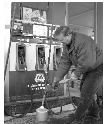
A field metrologist ensures gasoline sold in the Upper Peninsula meets performance standards.
