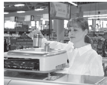
A field metrologist verifies the accuracy of a counter scale at a market deli. Ensuring fairness in food purchases benefits all Michigan consumers.
