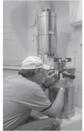
An MDA laboratory metrologist verifies the accuracy of a five gallon test measure used to inspect gasoline pumps across the state.
