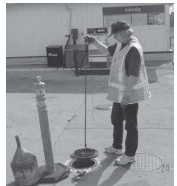
A field metrologist checks a station's gasoline storage tank for water. Station operators must ensure that consumers do not purchase fuel contaminated with water.
