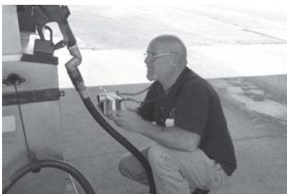
A senior Weights and Measures inspector makes a video record of the interior of a commercial measuring device. Inspections are key to determining if devices are of proper design and adequately maintained.
