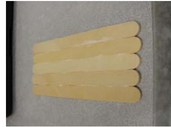
Picture C edge to edge is not laminating. This is acceptable.
