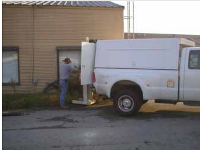
Geoprobe Vehicle Used for Soil Sampling
