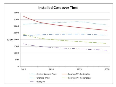
Figure ES-1. Renewable technology projected installed costs through 2030, in dollars per kilowatt.
