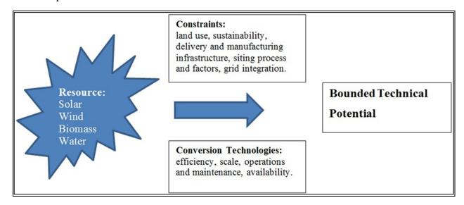
Figure 1. Bounded technical potential, showing the relationship constraints and conversion technologies.
