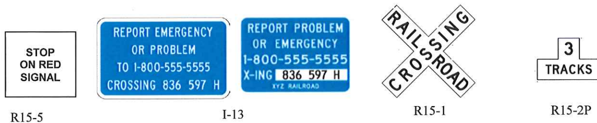
Figure 11: STOP ON RED SIGNAL sign, ENS signs, Crossbuck sign, and Number of Tracks sign
