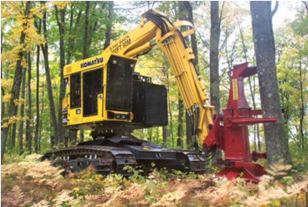
Figure 22. Tracked Komatsu XT Series Feller-Buncher.
