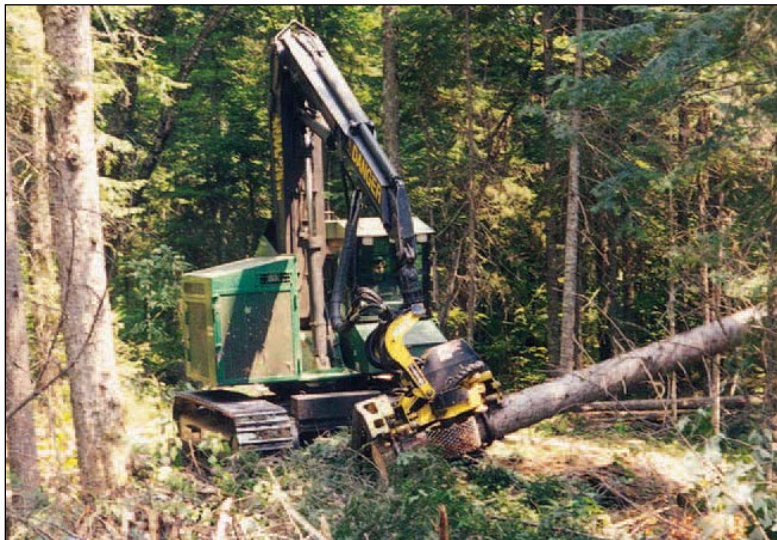
Figure 3. A Tracked Harvester with Extendable Boom.
