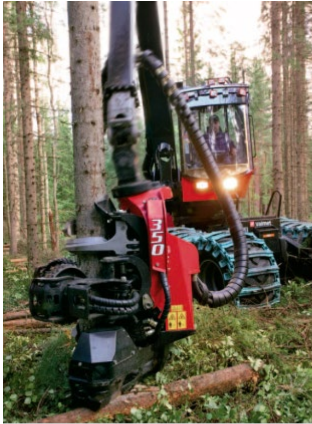
Figure 24. Cut-to-Length Harvester-Processor with Tracked Wheels.
