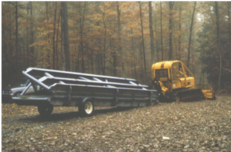
Figure 19. A Portable Folding Metal Bridge.
