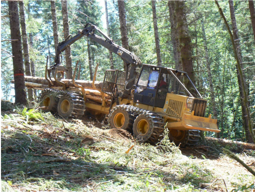
Figure 27. Caterpillar 574 Forwarder with Tracked Wheels.
