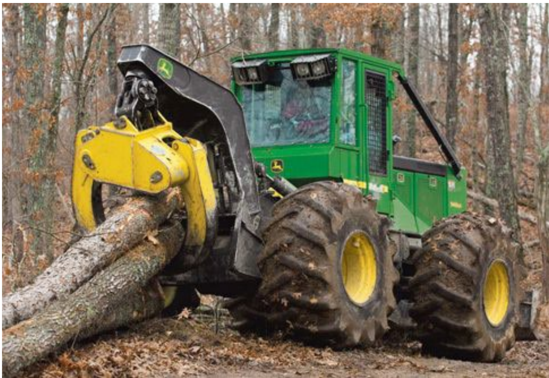
Figure 26. John Deere 548G-II Grapple Skidder with High Floatation Tires.
