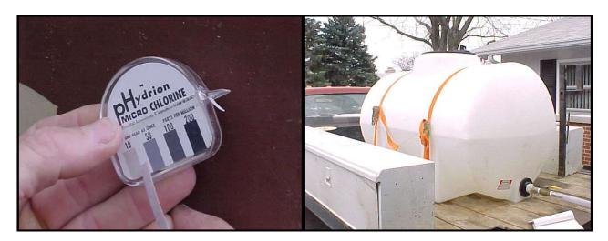
The drill water must be transported in a clean, sanitary container. Water transport tank outlets should allow for complete drainage of the tank. Water trucks/tanks should be cleaned occasionally to remove accumulated debris and mineral deposits.
