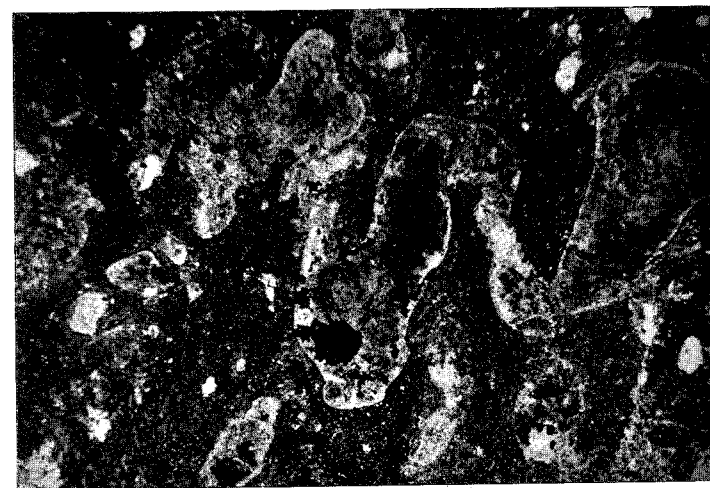
B. SUPERIOR LODGE, HOUGHTON MINE. PHOTOMICROGRAPH X 10. THIS SECTION SHOWS COARSE PARTICLES OF NATIVE COPPER IN LARGE AMYGDULES. IN THE DARK GROUND MASS THERE ARE NUMEROUS FINE PARTICLES OF METAL. THE LACK OF CRYSTALLINE STRUCTURE IN THE GROUND MASS IS NOTEWORTHY.
