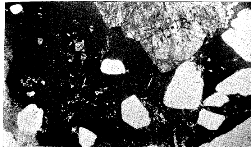
A. CALUMET CONGLOMERATE, CALUMET AND HECLA MINE. PHOTO-MICROGRAPH X 12. THIS IS A TYPICAL SECTION OF THE QUARTZ PORPHYRY OF THE CALUMET CONGLOMERATE SHOWING NUMEROUS CLEAR CRYSTALS OF QUARTZ IN A NEARLY OPAQUE FELSITE GROUND MASS. THE QUARTZ PORPHYRY PEBBLES CONTAIN SUCH NUMEROUS RED PARTICLES THAT THE GROUND MASS IS TRANSPARENT ONLY IN VERY THIN SECTIONS.
