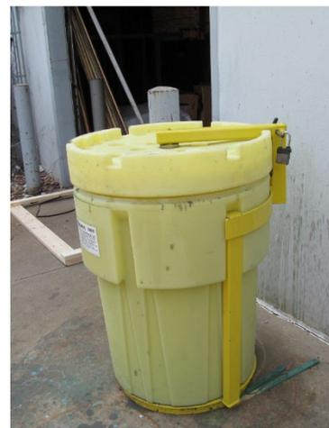
Single drum lockable secondary containment with squirt control
