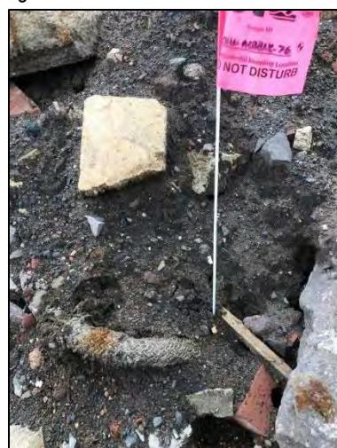
Photo 12: Rope gasket sampled as CHLL-ASBBLK76 in waste pile WP-27. Photo taken on 10/23/2017.
