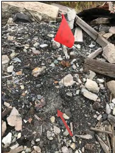
Photo 7: Suspect asbestos containing material (thermal system insulation). Photo taken on 8/21/2017.
