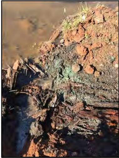
Photo 7: Green, copper material observed in test pit near Container #4 excavation site. Photo taken July 11, 2017.
