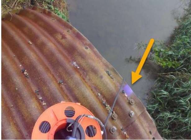
Figure 2. Mark on culvert for determining the relative water level. Measurements are from this point to the water's surface and were recorded on each sampling visit.
