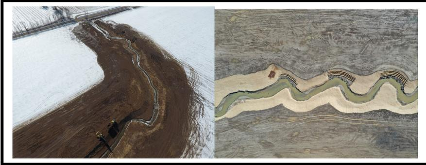
**Project aerial view: Most project areas involved streambank stabilization, re-contouring, two stage ditching, and other BMPs to counteract erosion.**
