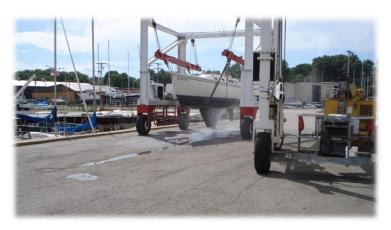
Using a high pressure wash system may eliminate the need for detergents and can reduce the volume of water used. In addition, if detergents are not used, an oil/water separator may be used to remove insoluble oils and sediment. However, this water will still need to be handled using the options previously described.
