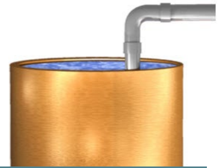
Typical Cross-Connection - Submerged Inlet
