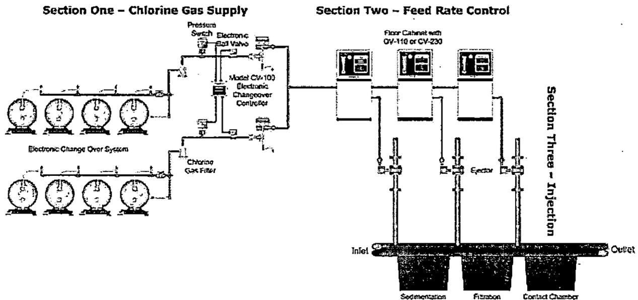
**Typical:** Gas chlorination systems follow a modular design principle. As seen in Figure 1 above, the gas chlorination equipment can be divided into three sections starting from the chlorine gas containers and ending at the ejectors as follows:
