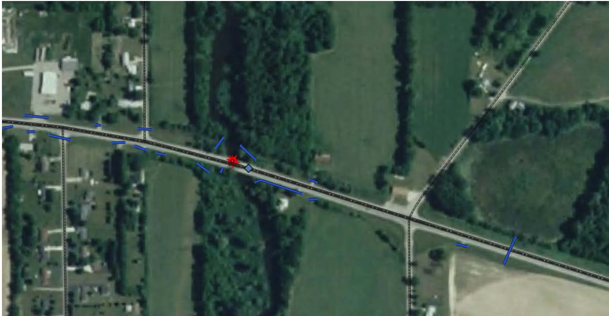
Figure 4: False positive new MDOT culvert shown by red star icon. MDOT bridge shown as blue diamond, MDOT culverts shown as dark blue lines
