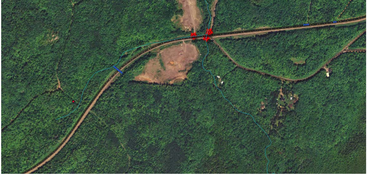
Figure 7: Potential new MDOT culverts shown as red stars. Known MDOT culverts shown as dark blue lines, other stream crossing surveys shown as red circles.
