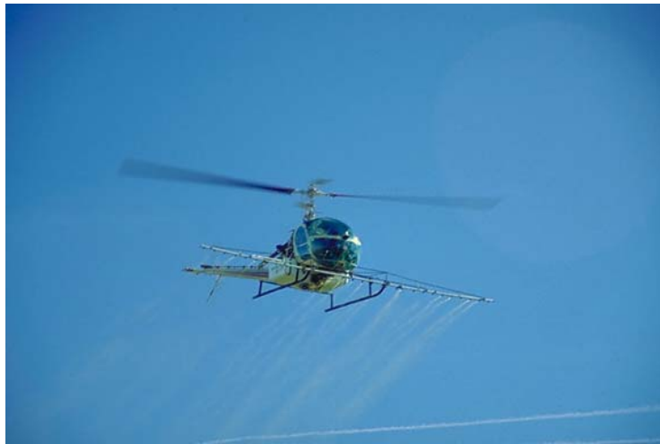
A Hiller helicopter in flight using a boom sprayer. Photo: 1999. M.J. Weaver; Virginia Polytechnic Institute and State University http://pesticidepics.ext.vt.edu/view_photo.php?set_albumName=album02&id=AA002
