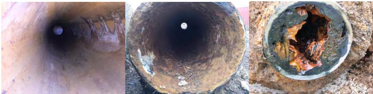
Hydraulic models commonly use the Hazen-Williams method of calculating friction loss in pressurized pipe applications. The pipe roughness coefficient, or C-factor, is adjusted to reflect the varying roughness within pipes.
