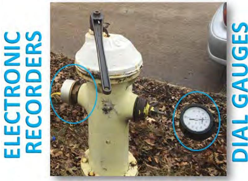
Arcadis maintains dial gauges and electronic recorders. The electronic recorders are predominately utilized for model calibration. In addition to pressure recorders, the apparatus used to measure pitot pressure can be a straight-tube pitot device with varying orifice diameters or a rotatable diffuser with integral pitot assembly.
