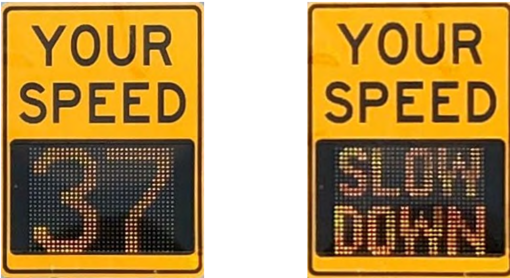
Figure 3. Dynamic radar speed feedback sign displaying example feedback messages
