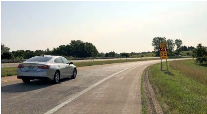
b. DSFS 255 ft Upstream of Curve (with 30 mph Advisory Speed Panel)
