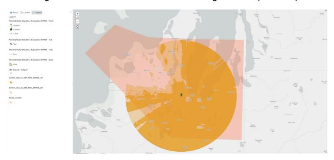
Figure 115: Indicative Radar Surveillance Coverage in Area 3 (500ft AGL)
