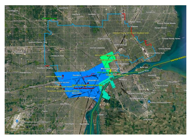
Figure 105: Existing (blue) and Proposed (red) Fiber Network for Areas 1 and 2 (with overlaid corridors)
