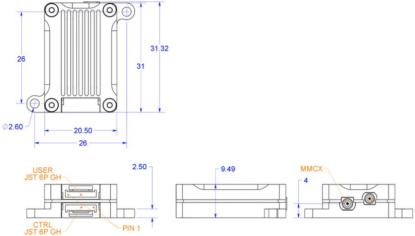
(sUAS). Figure **97** illustrates the mechanical specification of the ARS, with measurements provided in millimeters.
