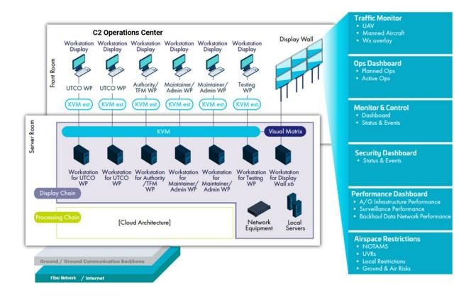
Figure 81: Example C2 Workstation Networking
