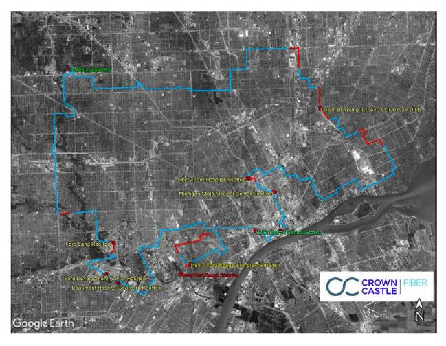
Figure 104: Existing (blue) and Proposed (red) Fiber Network for Areas 1 and 2 (with remote sites labeled)
