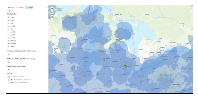
Figure 106: FAA Radar & ADS-B Coverage (500' AGL)
