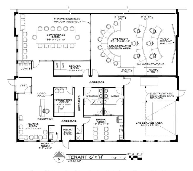
Figure 80: Example of Floorplan for C2 Center and Space Utilization
