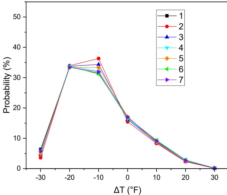
**Figure 5.8. Temperature gradient distribution (13" slab thickness)**
