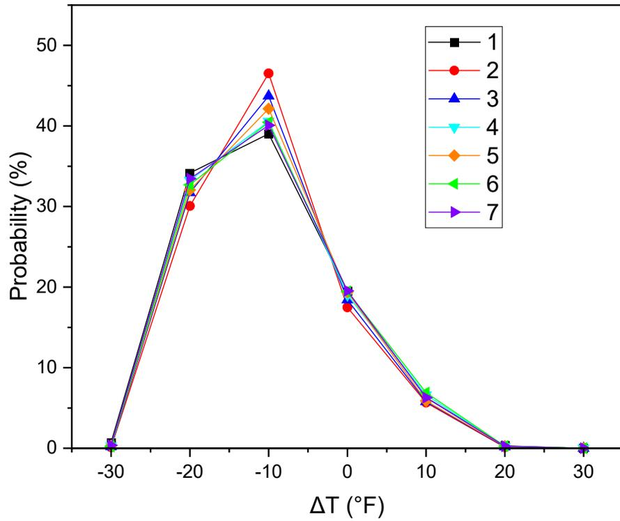
Figure 5.4. Temperature gradient distribution (6" slab thickness)
