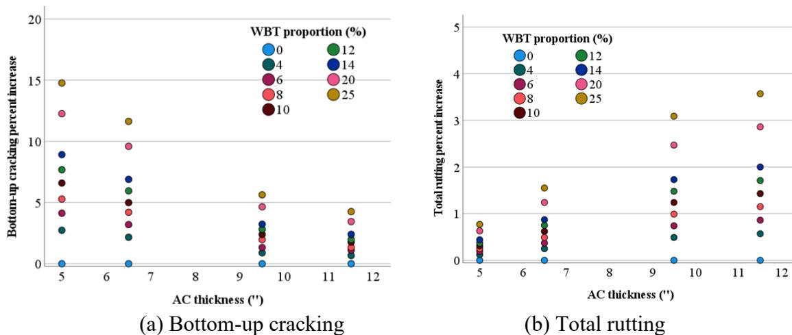
**Figure 4.26. Distress increase with the AC thickness**
