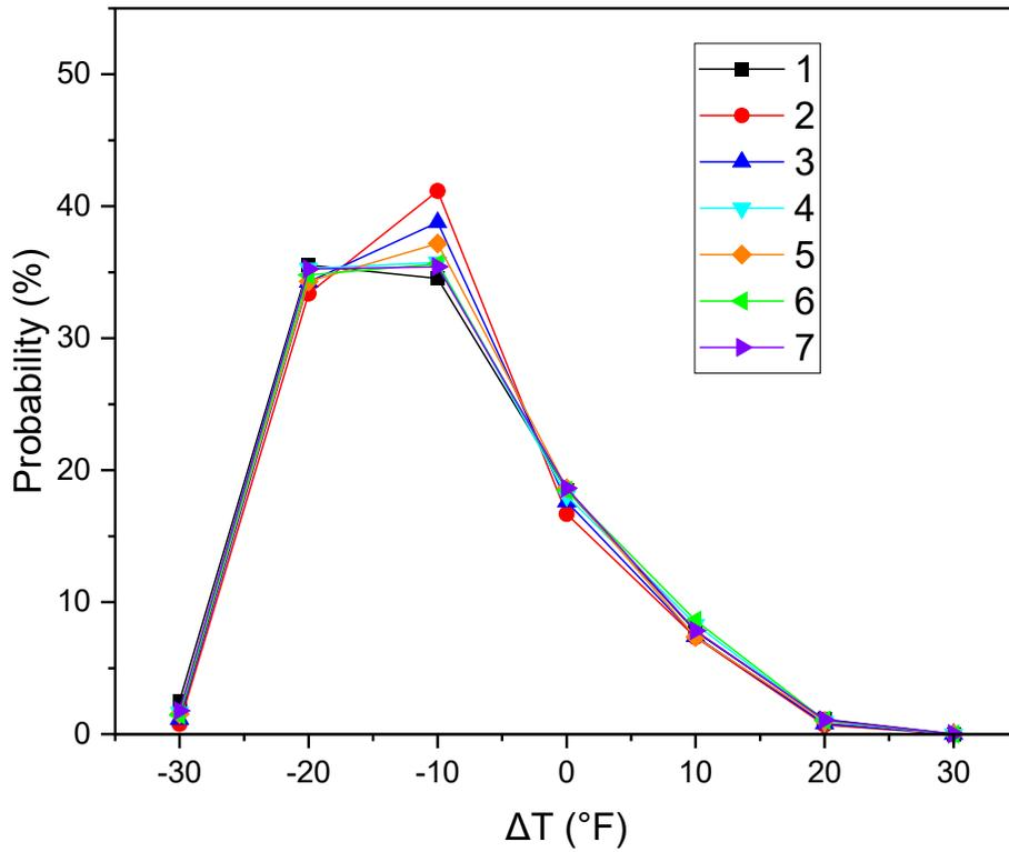
Figure 5.5. Temperature gradient distribution (8" slab thickness)
