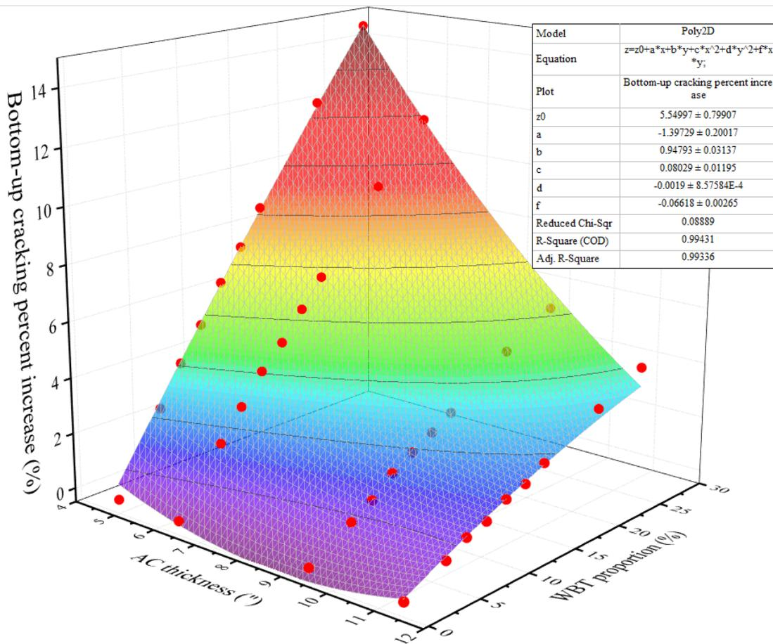
**Figure 4.27. Multiple regression of the bottom-up cracking distress**
