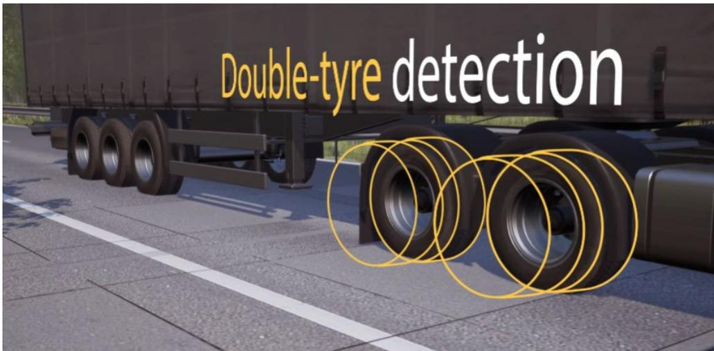
**Figure 6.6. Demonstration of WIM technology from OptiWIM**
