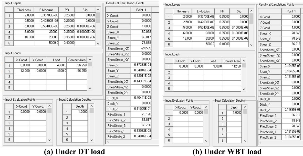
**Figure 4.12. JULEA examples for AC middle axial strain**
