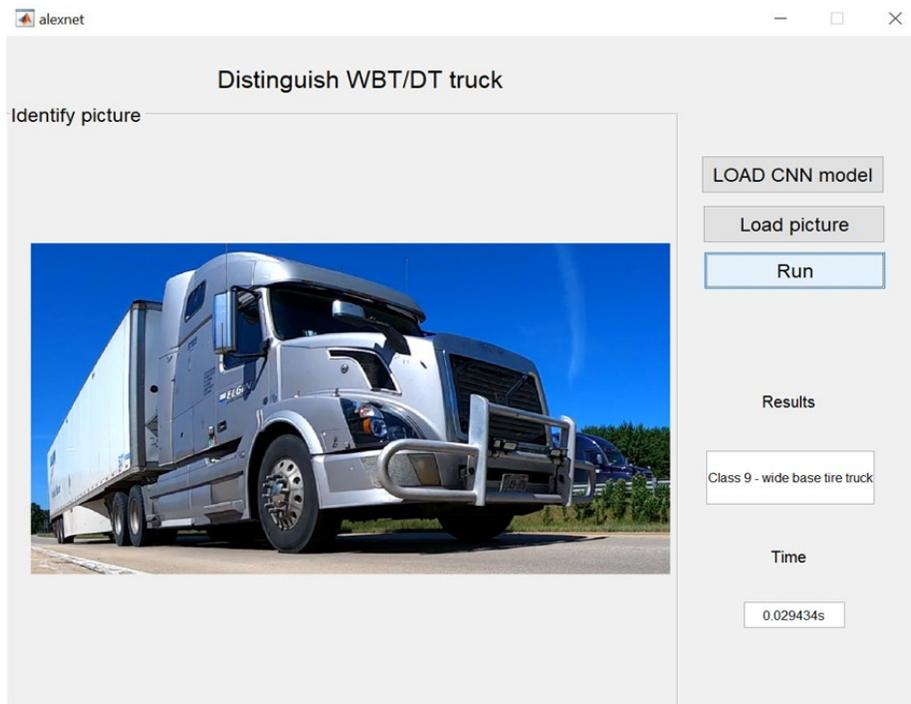
**Figure C.2. CNN App interface showing WBT truck**
