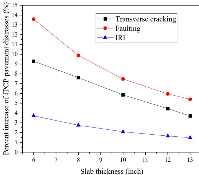
**Figure 5.41. Distress increase under 25% WBT load for different slab thickness structures**
