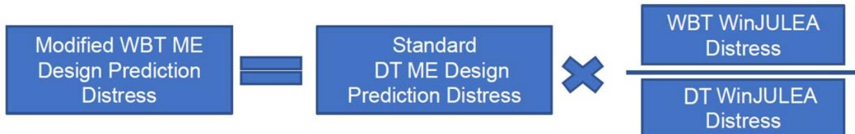
**Figure 4.29. The process of modifying the design considering WBT impact**
