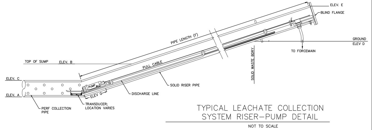
TYPICAL LEACHATE COLLECTION SYSTEM RISER-PUMP DETAIL
