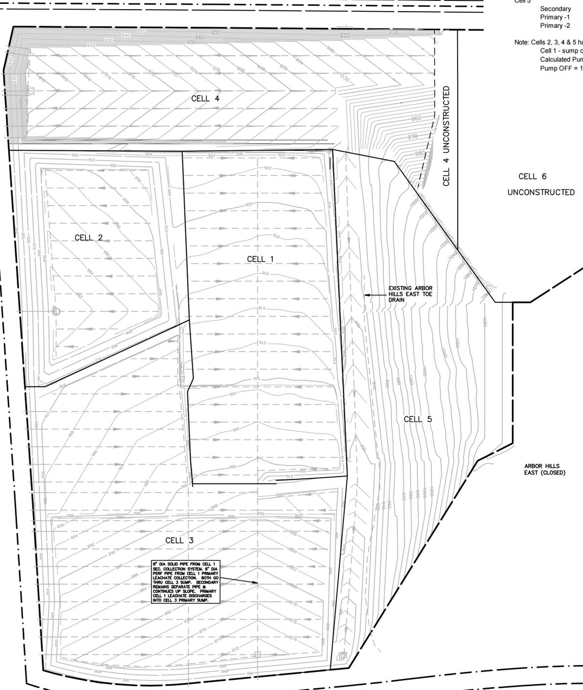
8" DIA SOLID PIPE FROM CELL 1 SEC. COLLECTION SYSTEM. 8" DIA PIPE FROM CELL 1 PRIMARY LEACHATE COLLECTION. BOTH GO THRU CELL 3 SUMP. SECONDARY REMAINS SEPARATE PIPE & CONTINUES UP SLOPE. PRIMARY CELL 1 LEACHATE DISCHARGES INTO CELL 3 PRIMARY SUMP.
