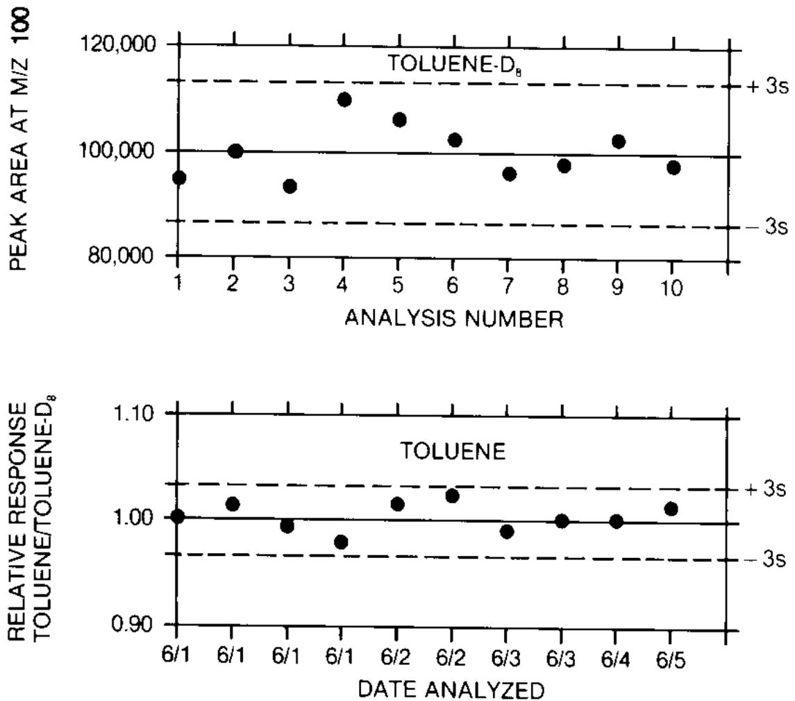
**FIGURE 8** Quality Control Charts Showing Area (top graph) and Relative Response of Toluene to Toluene-d<sub>8</sub> (lower graph) Plotted as Function of Time or Analysis Number
