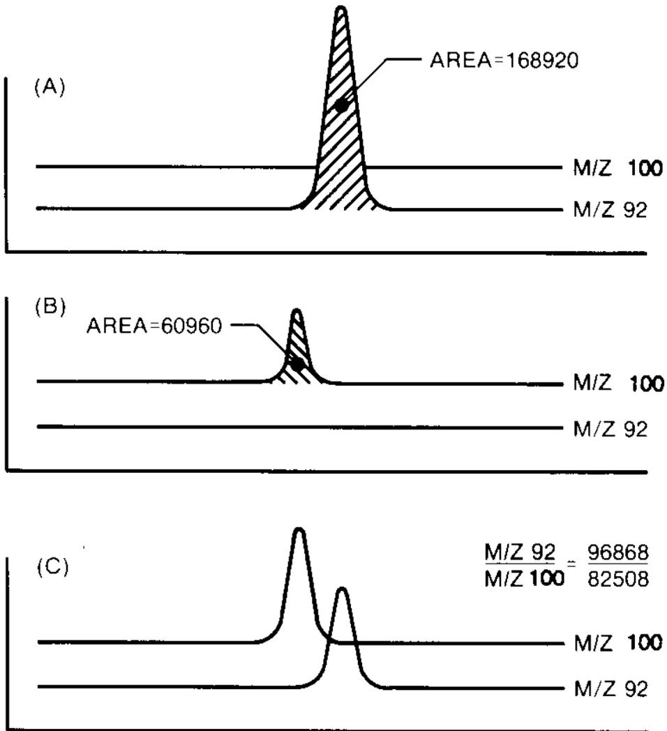
FIGURE 7 Extracted Ion Current Profiles for (A) Toluene, (B) Toluene-d<sub>8</sub>, and (C) a Mixture of Toluene and Toluene-d<sub>8</sub>
