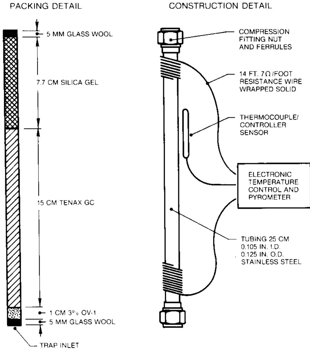
**FIGURE 3 Trap Construction and Packings**
