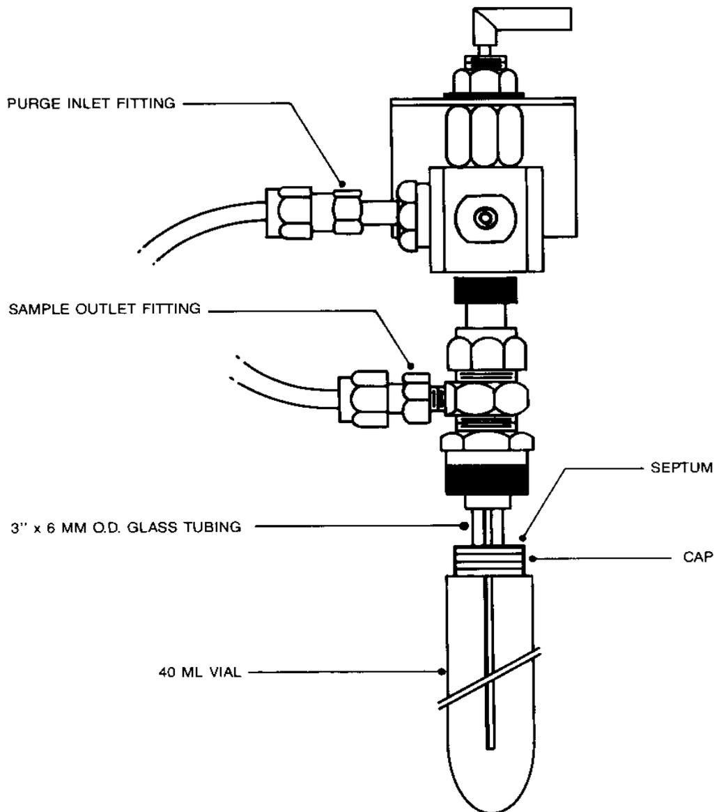
**FIGURE 2 Purging Device for Soils or Waters**
