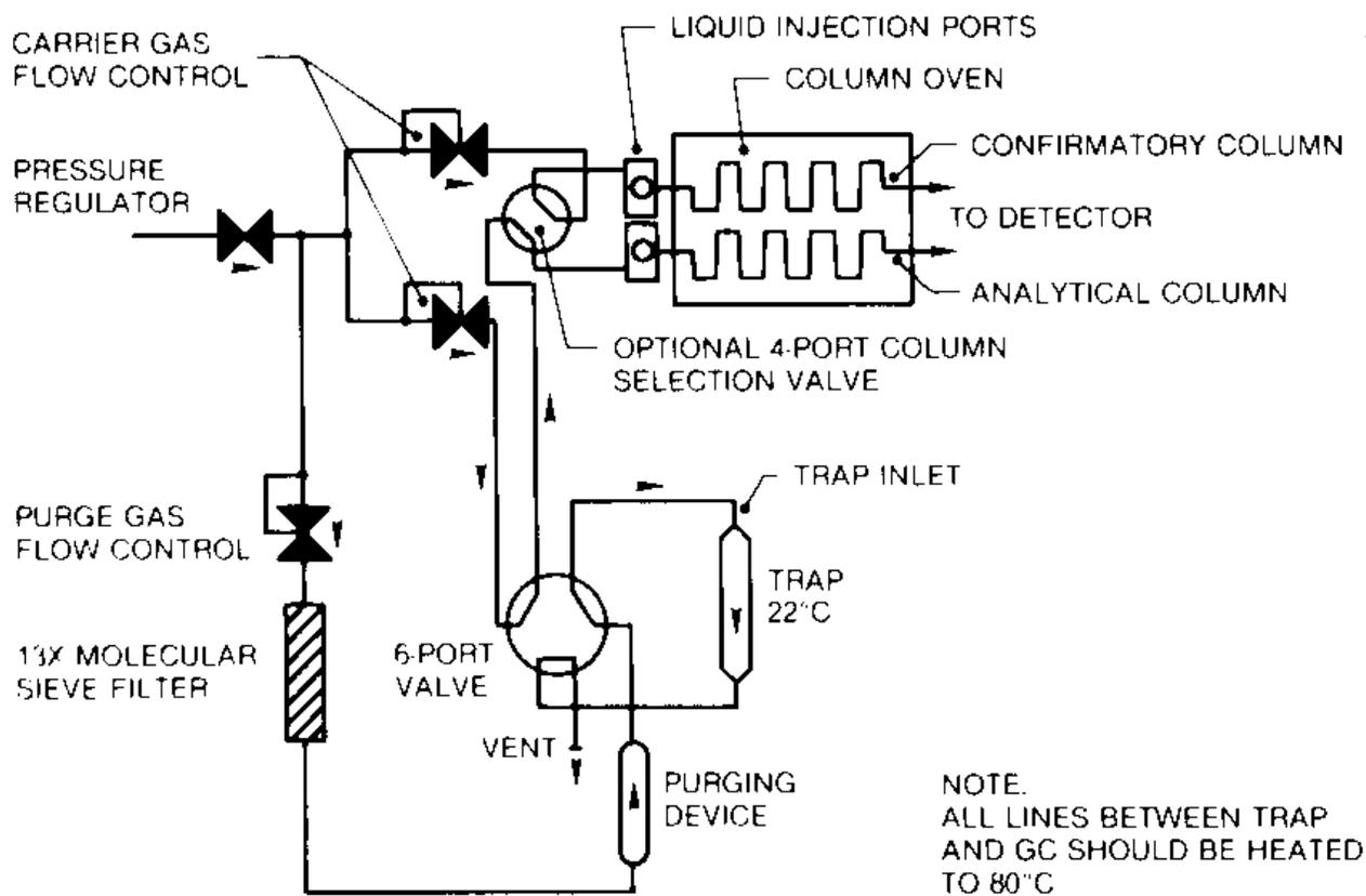
**FIGURE 4 Schematic of Purge and Trap Device--Purge Mode**
