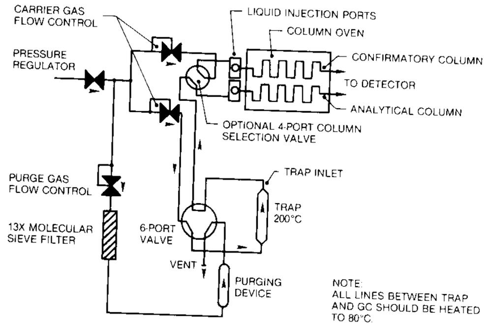
**FIGURE 5 Schematic of Purge and Trap Device--Desorb Mode**
