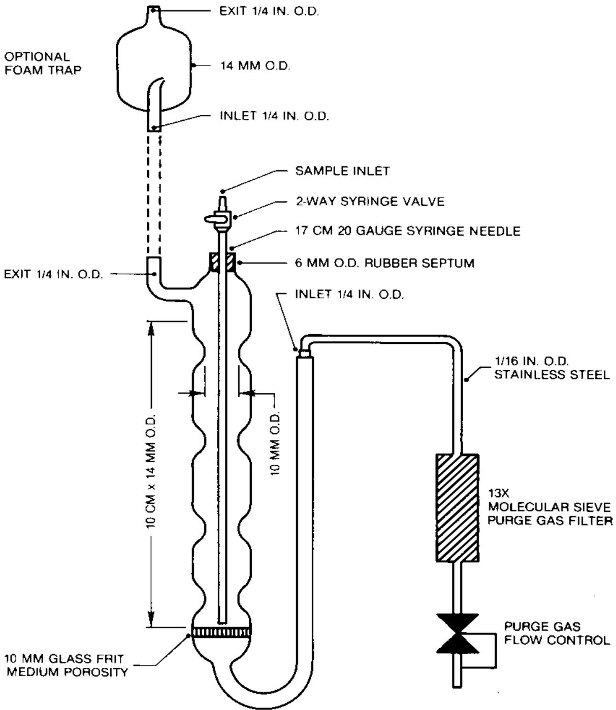
**FIGURE 1 Purging Device for Waters**
